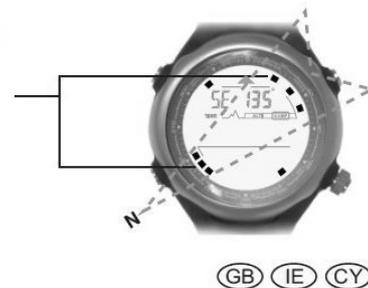
Example: finding north The symbol (■ ■ ■) can be regarded as the tip of an imaginary needle pointing towards north. The Symbol (■ ■ ■) represents the "tail" end of the needle pointing towards south. Regardless of the orientation of the compass. north and south is always easily identified with the symbols (■ ■ ■) and (■ ■ ■).
